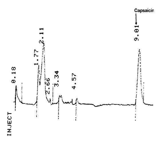
Figure A-1. HPLC chart of standard: injection of 10µl of 0.3µM capsaicin in acetonitrile. Capsaicin peak at approximate timepoint of 9 minutes.
