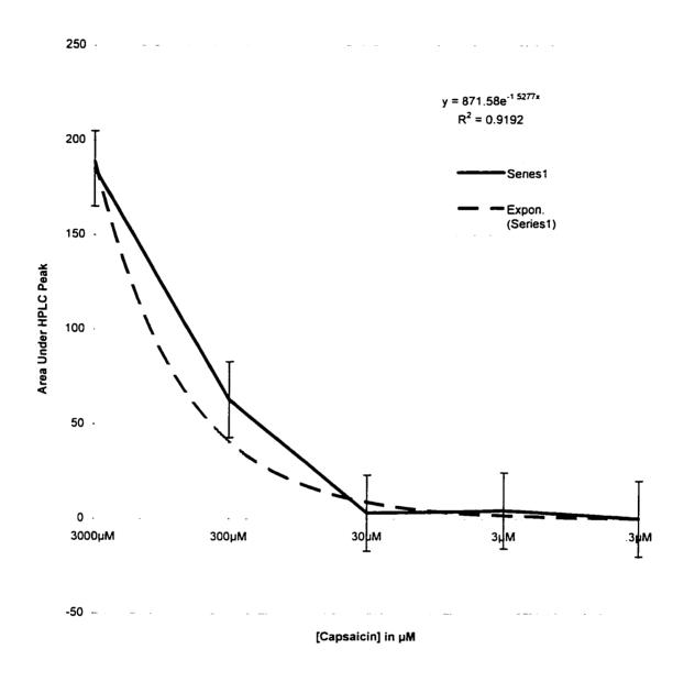
Figure 3. Standard curve of capsaicin concentration vs. area under HPLC peak (± SEM). Series 1 = standard curve. Expon (series 1) = theoretical curve.
